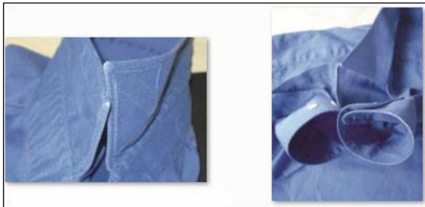
Fig.7.Result of insufficient abrasion resistance
